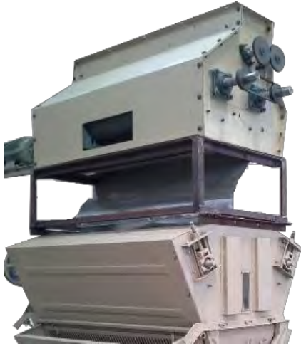
Fig. 6. Combined feeder (M3)
