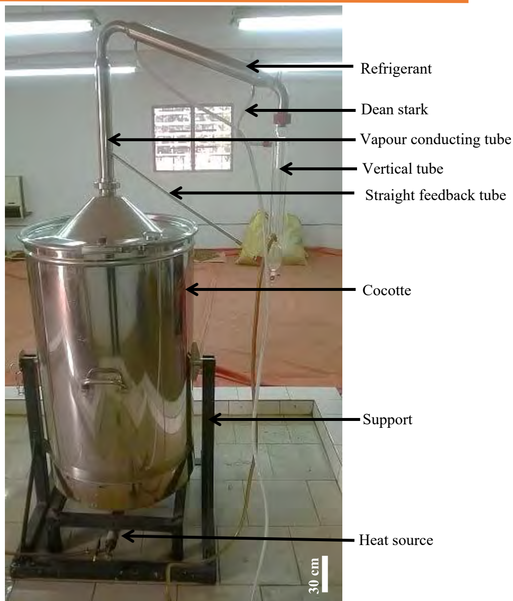
Figure 6. Clevenger apparatus (stainless steel) for the extraction of essential oils
