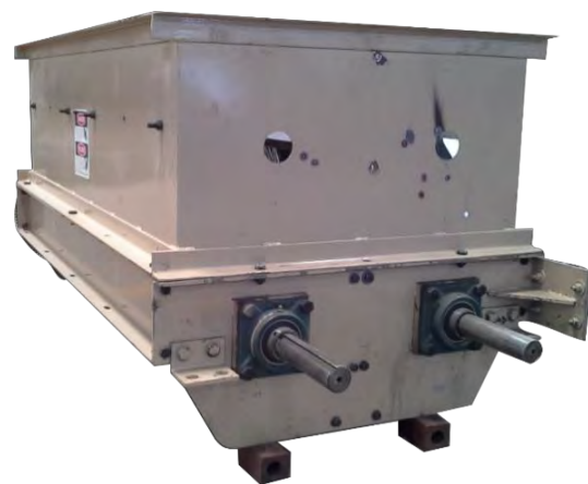
Fig. 5. Saw band cylinder feeder (M2)
