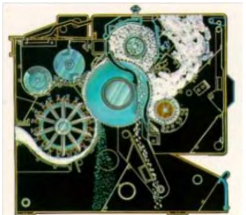
Pic 2: Working Principle of Brush Type Saw Gin
