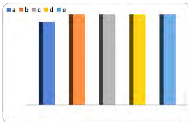
Figure 5. Tensile strength (CN/Tex) of cotton yarns: (a) Raw cotton yarns; (b) scoured cotton yarns; (c) dyed with natural dye; (d) dyed with reactive dyes ; (e) dyed with basic dyes
