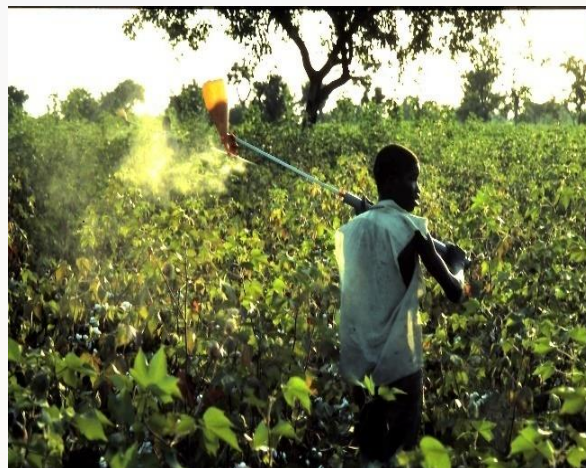
Fig. 1b Rotary atomiser ULV sprayer used in Cameroon.
