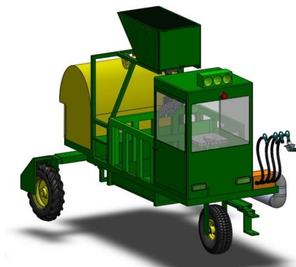
Fig 1- 3D model of small cotton harvester created by Solidworks softwear
