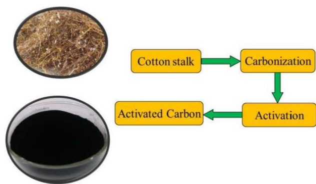
Fig. 1: Methodology adopted for preparation of activated carbon from cotton stalk
