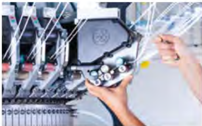
Figure (2): Drafting Unit.
