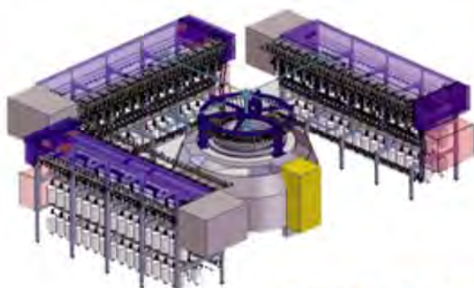
Figure (3): The Terrot direct spin-knit "Corizon"
