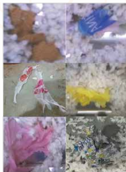
Figure 4. VIPR system during operation shown above gin stand (left) and images of contamination detected and removed from the process stream before the cotton entered the gin stand (right).
