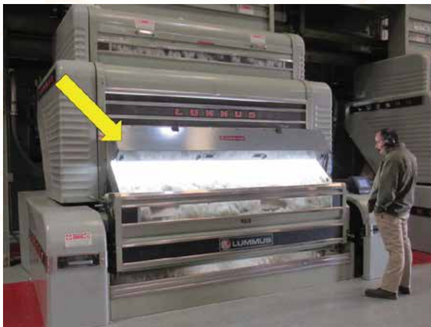
Figure 4. VIPR system during operation shown above gin stand (left) and images of contamination detected and removed from the process stream before the cotton entered the gin stand (right).
