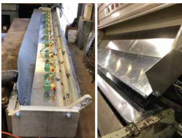
Figure 2. The PIDES air ejection solenoids under lower feeder apron (left) and top view showing the air knife ejection device at the end of the feeder apron (right).
