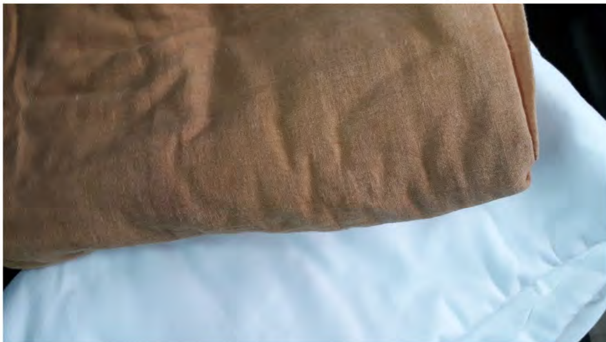
Figure 1. Cotton fabrics (below) treated with Nano silver (above). The colour is due to the surface plasmon effect of Nano silver
