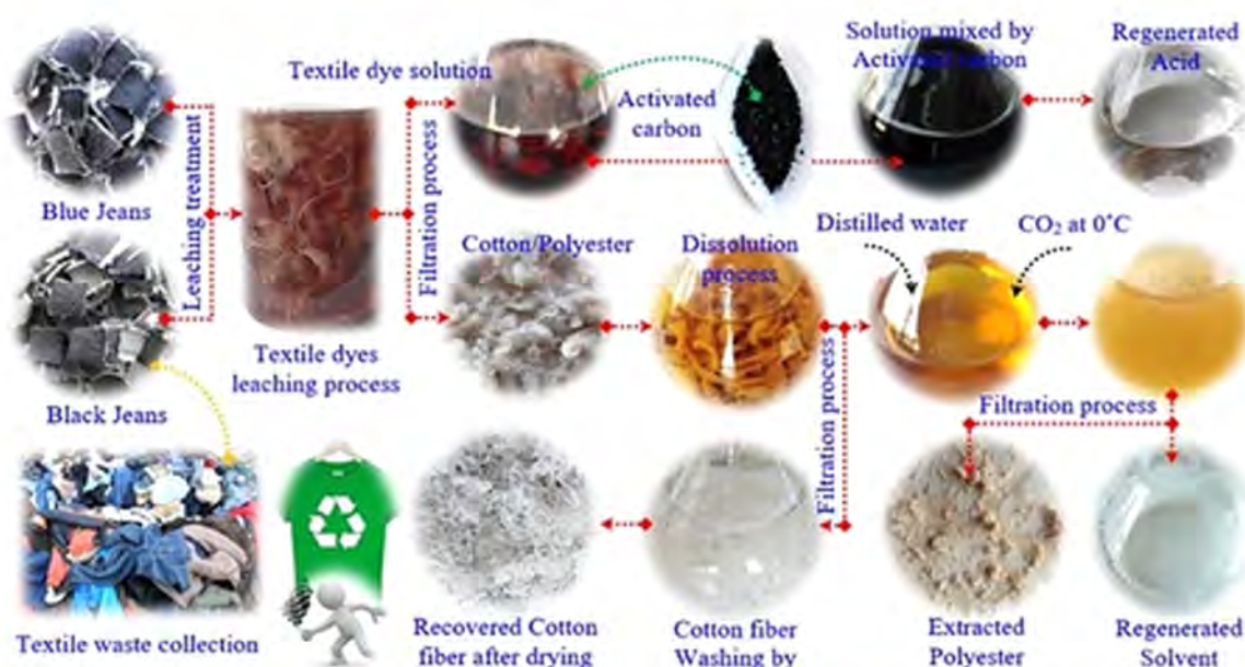
Fig. (2): Waste jeans separation flowchart
