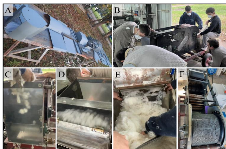
Figure 5. Images of the construction process and commissioning of the mini ginner. Treatment and painting process of individual parts (A), initial ginning tests (B), rear viewer of the machine where raw cotton is loaded (C), top viewer showing the saws in the ginning process (D), clean fiber output area (E), and top view of the internal duct system for fiber passage (F).
