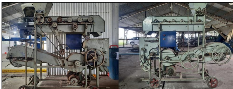
Figure 3. Old ginner surveyed to initiate the design and adaptation process of the machine proposed in the project, viewed from both sides.
