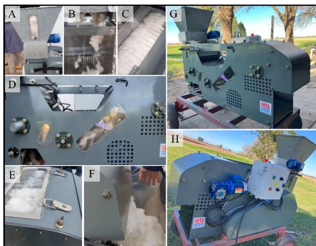
Figure 7. Images of the final machine in operation. Entry of raw cotton into the loader (A), rear viewer where the fiber falls into the saw system (B), ginning process (C), side viewers showing the passage of fiber (D), viewer from the top of the condenser (E), and exit of clean fiber from the front (F). Side views of the completed mini ginner (G-H).
